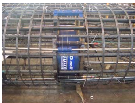
O-cell assembly made at Rom-Tech's cage fabrication facility in Sheffield
