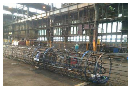
O-cell assembly made at Rom-Tech's cage fabrication facility in Sheffield
