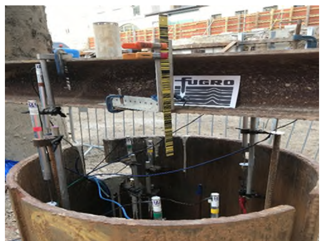
O-Cell® test in progress. The steel beam is for reference only
