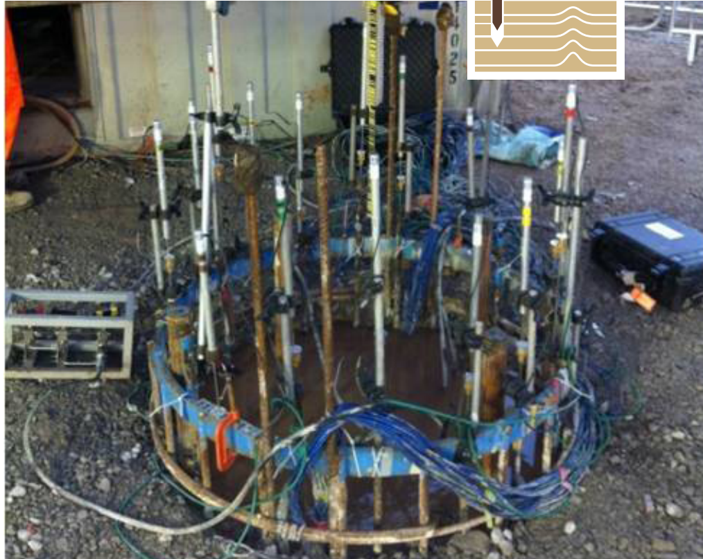
O-cell pile testing in progress to 57MN
